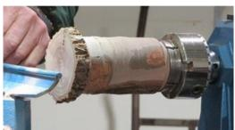
Remove the tailstock and turn the end of the piece square.
