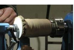
Ron showed his method of supporting the piece by using a circular piece of MDF with a small centre hole. This simple
