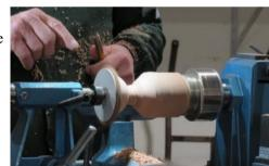
Once the desired thickness is achieved, start to turn the stem. Ron decided to have a feature between the cup and the stem. Complete this before moving onto the stem
