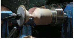
Working from the feature towards the headstock start turning down to the desired diameter of
