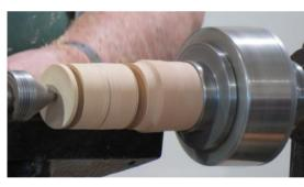
Turn tenons on both ends, one to fit in a chuck.
