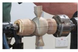
Remove the piece and use two cup chucks to hold the partially finished sphere at 90° to what it was. Ron showed us a cup to fit over his live centre and another to fit into a scroll chuck.
