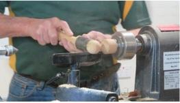
Hold the piece in a jam chuck to remove the tenon nib. (Ron noted that there is not much to hold a sphere in a jam chuck so use sandpaper to do this, or be very light-handed with a chisel
