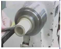
12. Cut an outside rebate to be used as a jam fit for the base of the box. Shape the base to the desired thickness to the drilled hole. DO NOT PART OFF
