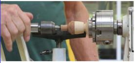
13.Jam fit the top to the base as illustrated. The shaped base can be seen in profile.
