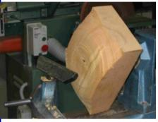
Start shaping the underside of the dish just like starting any bowl. Use a bowl gouge with a pulling cut. This is pulling the gouge
