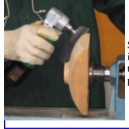
Sand the underside of the dish. The foot can adjacent area can be sanded while the part is rotating BUT sand the wings while the blank is stationary. If you try to sand while the part is rotating, the leading edges of the wings will become rounded as the sanding pad vibrates in and out of the shadow (gap between the blank as it rotates.).
