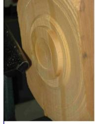
Start removing the waste around the foot of the dish
