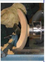
When the wall thickness is as required, sand the inside of the dish. The centre area can be sanded while the part is rotating BUT sand the wings while the blank is stationary. If you try to sand while the part is rotating, the leading edges of the wings will become rounded as the sanding pad vibrates in and out of the shadow (gap between the blank as it rotates.).
