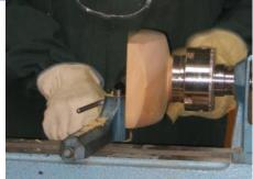
Continue removing moving waste. Stop the lathe
