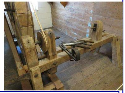
I was impressed with the size of the fly wheel which was about 1.5 meters diameter and the rope pulley instead of a belt. Nobody there could tell me how the lathe was powered.
