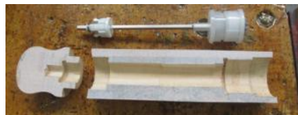
Cross section of grinder with mechanism
