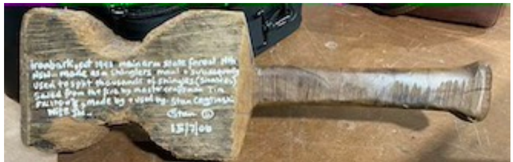
"Ironbark cut 1992 main arm state forest Nth NSW Made as a shinglers maul & subsequently used to split thousands of shingles (shakes) Saved from the fire by the master craftsman Tim Skilton's wife Jac Made & used by Stan Cegliaski Stan 15/7/06"
