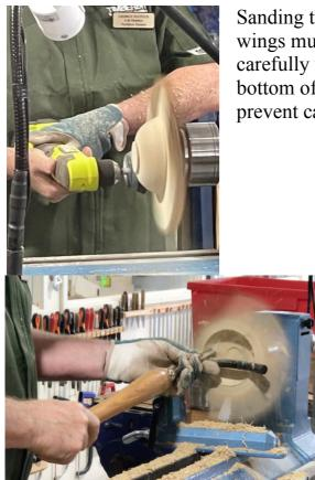
Sanding the spinning wings must be done carefully using the bottom of the disc to prevent catching.
