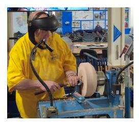
Tim, bravely, demonstrated his bowl saver. It is an interesting tool for carving out the inner part of a large piece of wood to create smaller bowl blanks. It is best used on wet timber. Tim brought in his one horsepower lathe (735.5 Nm) to do the demo and it was working quite hard.
