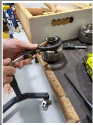
Barry Warneke also demonstrating the use of a tenon-making tool that he acquired in a collection of second-hand tools.
