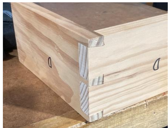
A completed dove-tail joint.
