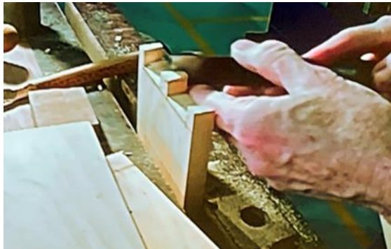
A chisel completes removal of waste
