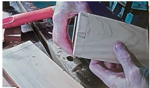
The joint is assembled to check for fit.
