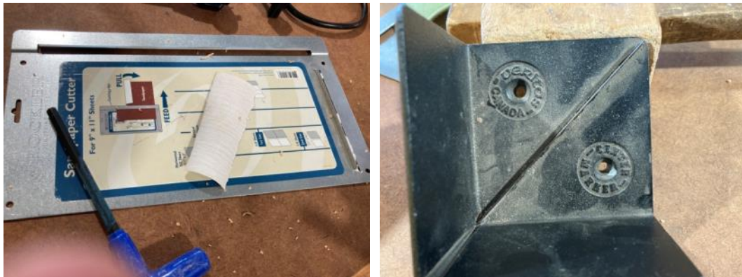
The sandpaper cutter (left) and the centring marker with 45 degree blade
