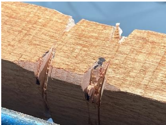
The first cuts on either side of centre
