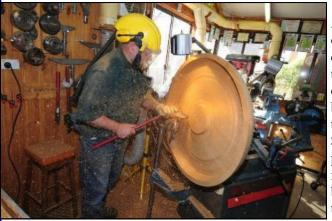
After reversing the blank onto the large Vicmark chuck, I fitted a bowl saver to the lathe in preparation to core out the centre of the blank. I then had second
