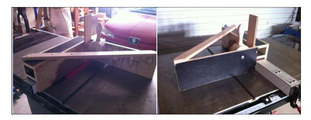
The tenoning jig to cut the joinery for the drawers.
