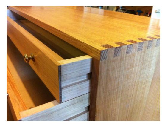
Detail of the joints used for the carcass of the drawers
